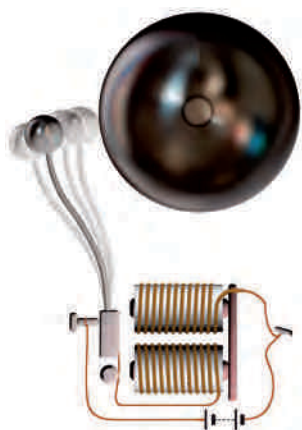
Fig. 10. 20 Circuit of an electric bell
