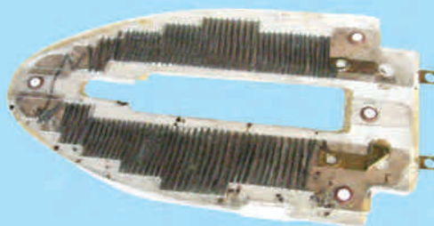
Fig. 10.11 Element of electric iron
